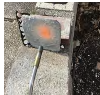
Fire Stop meets or exceeds international specifications for passive fireproofing in public structures and infrastructures to control "hot" areas. Tests on 1/2" to 3/4" samples at 2400°F for 4 hrs showed the back side never exceeded 800°F.
